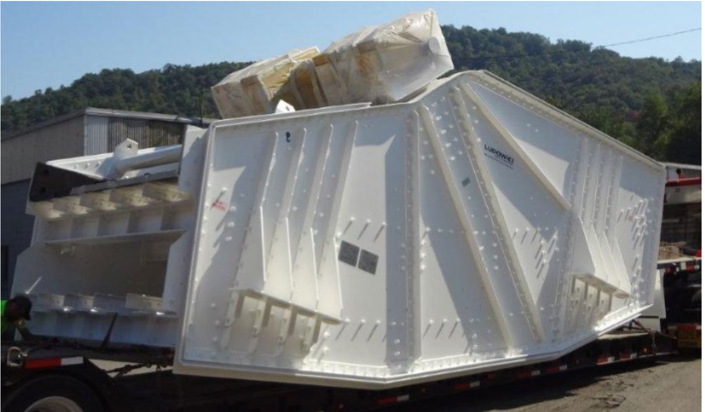
Figure 4: Ludowici double deck Banana screen
