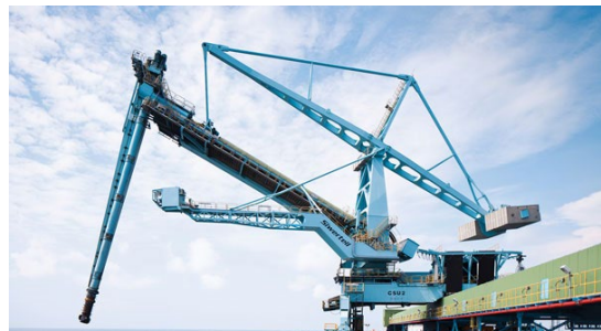
Figure 10: Dockside Screw Rail Mounted Unloader (photo courtesy of Siwertell)
