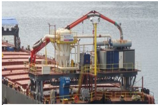
Figure 9: Floating Storage Rail Mounted Unloader (Photo courtesy of VAN AALST Bulk Handling)
