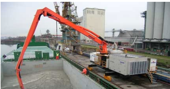
Figure 11: Pnuematic Rail Mounted Unloader (photo courtesy of FLSmidth)
