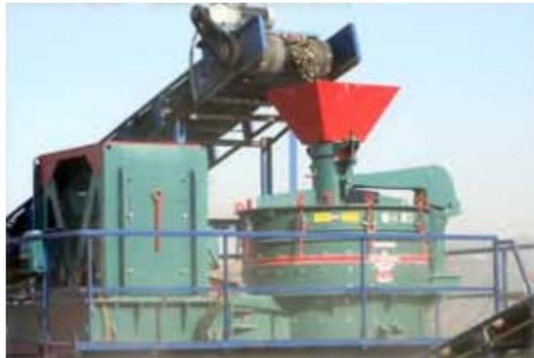
3. Most of the waste sand is normally dumped at the end of the crushing plant. The addition of a closed circuit at the end of the crushing plant to convey this waste product to a properly sized VSI can de-cluster additional sand grains and increase the product yield. This VSI works together with a screen to separate the final product.
