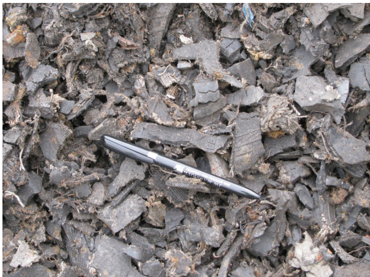
RDF FUEL USED BY A CEMENT PLANT
