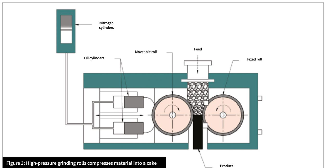
Figure 3: High-pressure grinding rolls compresses material into a cake
