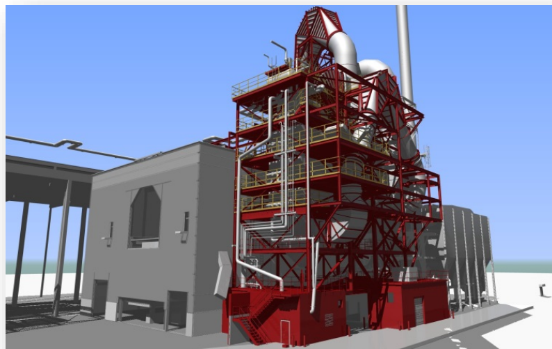
Figure 3 – Visualization of a Clinker Cooler in a cement plant
